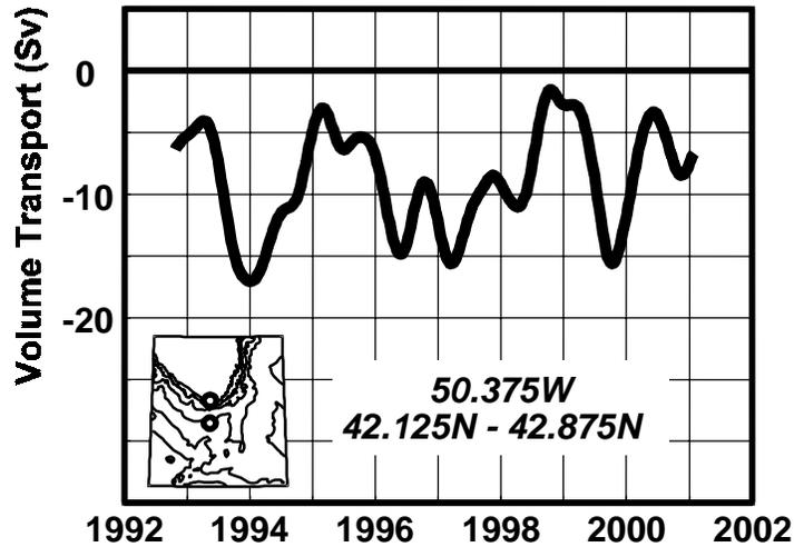
**Figure 5.** Westward volume transport for temperatures between 3°C and 5°C based on TOPEX/POSEIDON sea level measurements near 50°W from September 1992 to January 2001. The inset map shows the locations of the sea level time series used to construct the transport estimates.
