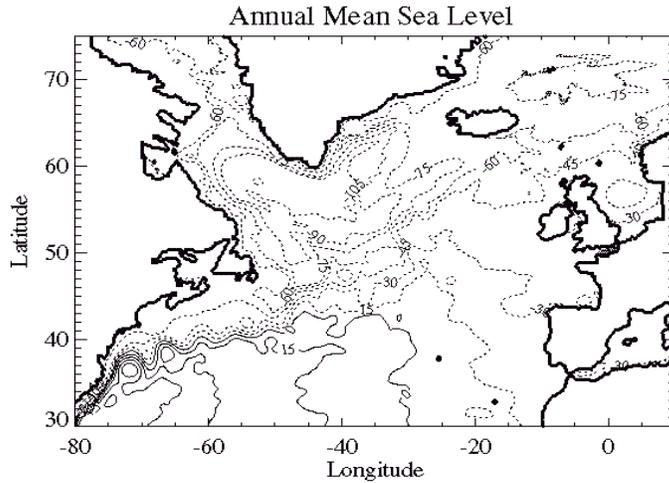
**Figure 2.** Mean sea surface height simulated by a 1/6 degree Atlantic Ocean general circulation model of Chao et al. (1996).
