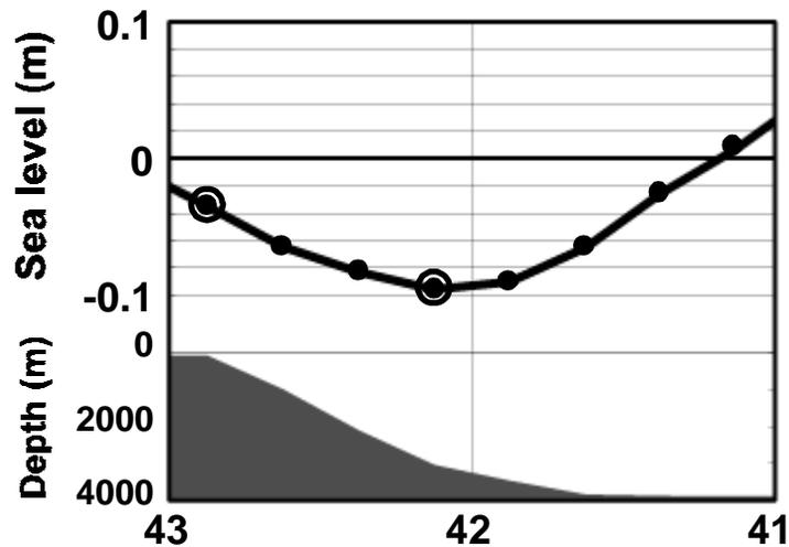
**Figure 6.** Temporally low-passed TOPEX/POSEIDON sea level anomaly along 50.375°W for May 24, 1996. The difference in sea level between the highlighted symbols is -0.06 m. This gives a volume transport of -14.8 Sv in Figure 5. A bathymetric profile is also shown.
